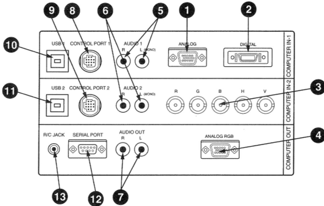
**1 COMPUTER INPUT-1 TERMINAL (ANALOG HDB 15-PIN)**
